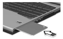
To remove the Smart Card press the Smart Card eject button (a) and remove the Smart Card (b) as shown in the illustration below.
